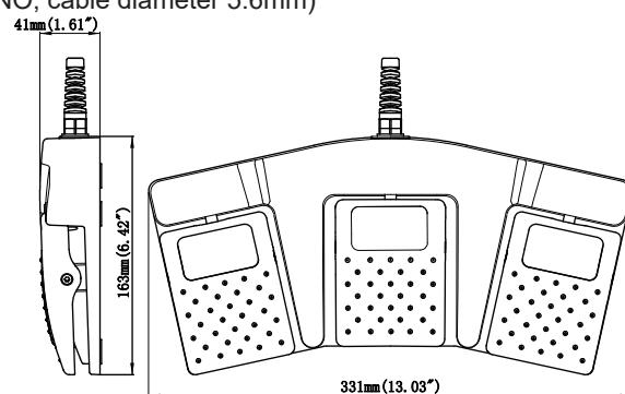
**FX-84-5-W-N-B2-H-26/7** (26AWGx7, PUR, coiled, 6x 1NO, cable diameter 5.3mm)
