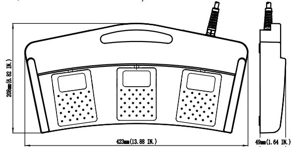
**FX-83-5-WP-N-2-20/4S** (20AWGx4, shielded, 2 meters, 2x 1NO, cable diameter 7.0mm)
