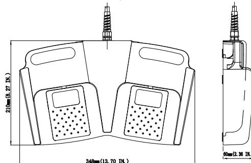
**FX-83-5-W-N-2-20/4S** (20AWGx4, shielded, 2 meters, 2x 1NO, cable diameter 7.0mm)
