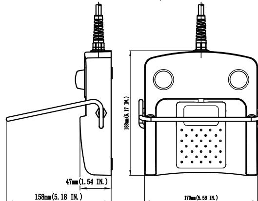
**FX-81-5-W-N-B3-H-2-22/5S-(L)** (22AWGx5, shielded, 2 meters, 2x 1NO, cable diameter 5.6mm)
