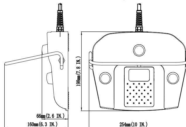
**FX-82-5-W-N-2-20/4S-(S)** (20AWGx4, shielded, 2 meters, 2x 1NO, cable diameter 7.0mm)
