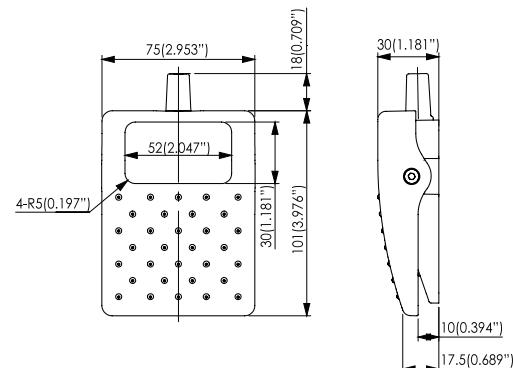
**FX-82-5-W-N-2-20/4S(S)** (20AWGx4, shielded, 2 meters, 2x 1NO, cable diameter 7.0mm, Compact Base)
